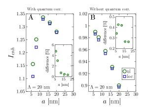
Fig. 1. Impact of strong coupling corrections on the photocurrent. (A) with and (B) without particle–substrate coupling. The lattice period is  $\Lambda = 20$  nm and various nanoparticle radii *a* are used. The insets show the difference between classical and nonlocal theory results.
