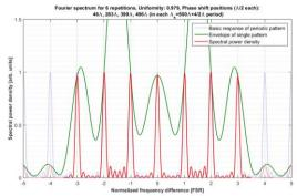
Fig. 2. 7-peaked phase-modulated grating design with flat envelope
