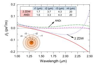
Fig. 1. Different designed dispersion profiles of the proposed Ge-doped fourlayer cylindrical silica fibers.
