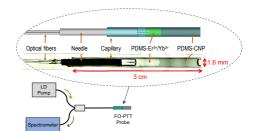
Fig. 1. Schematic representation (above) and actual image (below) of the fiber-optic photothermal (FO-PTT) probe. The probe includes a photothermal polymer composite for heat generation (PDMS-CNP) and a fluorescent compound for temperature measurements (PDMS- $\mathrm{Er}^{3+}/\mathrm{Yb}^{3+}$ ).
