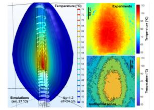
Fig. 3. Temperature profiles in the vicinity of the FO-PTT probe obtained through computer simulations (left) and experimental results obtained with laser-induced fluorescent thermometry (right).
