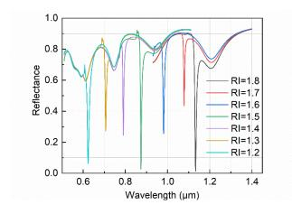
Figure 3: Reflectance spectra when different refractive index is being sensed.
