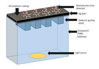
Figure 1: Structure of the biosensor.
