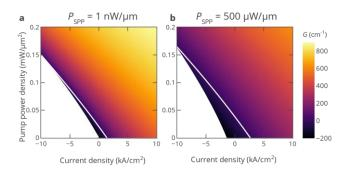
Fig. 2. SPP modal gain as a function of the pump current density and the optical pump power density calculated at low (1 nW/µm, panel a) and high (500 µW/µm, panel b) powers of the SPP signal. The white line in both panels corresponds to the regime of lossless SPP propagation.
