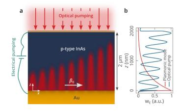
Fig. 1. (a) Schematic view of a planar plasmonic waveguide pumped both electrically and optically. (b) Spatial dependence of the electric energy density ( $w_E$ ) in the SPP wave and the optical pump laser beam.
