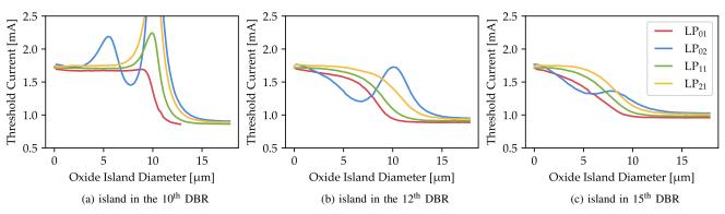
Fig. 1. Dependence of threshold current on the size of the oxide island for several locations in the DBR layers. The position of the island has a strong impact the qualitative behavior of the modes. Below the  $12^{th}$  pair, strong oscillations are visible. A rapid increase in threshold current can be observed for critical island diameters (10 µm and around 5 µm for the LP<sub>02</sub> mode).
