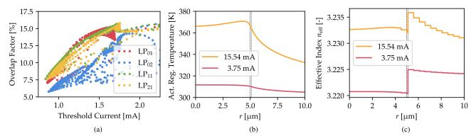
Fig. 2. The correlation between the overlap factor and the threshold current (a), temperature profile (b) and effective index distribution (c) in the active region for input currents of 3.75 mA and 15.54 mA.
