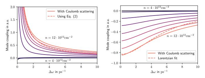
Fig. 2. Asymmetric (left) and symmetric (right) mode coupling terms shown as function of the frequency difference of the two longitudinal modes. Here one of the two modes is chosen to be at the gain maximum.
