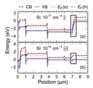
Fig. 3. Short-circuit band diagrams for (a) low and (b) high doping in the Si substrate. Potential barrier at Ge/Si interface is boxed. Ge interface layer doping is  $10^{17}$  cm<sup>-3</sup>, *TDD* = 0 cm<sup>-2</sup>.
