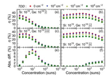
Fig. 5. (a)-(d) Triple-junction solar cell efficiency,  $\eta$ , vs. irradiance. Doping concentrations are indicated. (e), (f) Absolute efficiency gain obtained by increasing Ge interface layer doping from  $10^{18}$  to  $10^{19}$  cm<sup>-3</sup> for Si doped at (e)  $10^{18}$  and (f)  $10^{19}$  cm<sup>-3</sup>.
