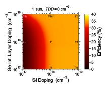
Fig. 2. Triple-junction solar cell efficiency at 1 sun vs. Si substrate and Ge interface layer doping, cell designs indicated.
