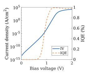
Fig. 2. The I-V curve showing SRH and radiative recombination dominated regimes. The IQE of the device starts to increase as radiative recombination starts to dominate, and stays over 97 % at biases above 1.2 V.
