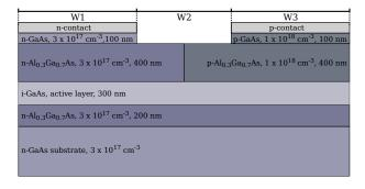
Fig. 1. Schematic structure of one period of the studied LHJ GaAs/AlGaAs DDCT LED.
