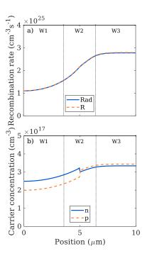
Fig. 3. (a) Radiative and total recombination rates and (b) the carrier concentrations within the AL as a function of lateral position at  $J = 100 \text{ A/cm}^2$ .
