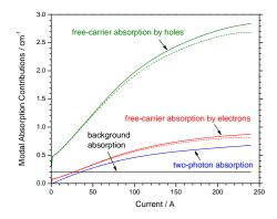
Fig. 2: Contributions of the different absorption mechanisms to the modal optical loss vs. current. Solid lines: full model. Dashed lines: free-carrier absorption without two-photon absorption.
