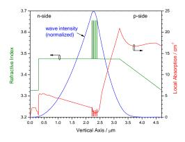
Fig. 1: Vertical profiles of refractive index, wave intensity (normalized), and local absorption.
