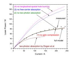
Fig. 3: Laser power vs. current as measured (+++) and as simulated with the full model (solid line). The dashed lines show the simulation results after subsequent removal of key mechanisms from the model.
