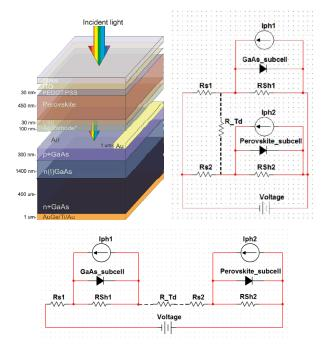
Fig. 1 Tandem device schematics (GaAs- perovskite tandem at short circuit regime); equivalent circuits of parallel and in-
