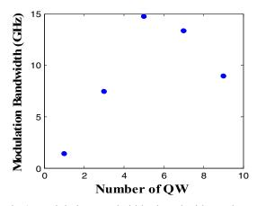
Fig.4. Modulation Bandwidth plotted with number of well
