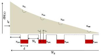
Fig.2: Schematic of carrier diffusion, quantum capture and escape in the MQW transistor laser
