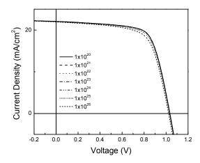
Fig. 3. Simulated J-V curves for different effective hole trap densities.
