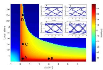
Fig. 2 SMSR for different wavelength interval and loss ratio. Insert : eye diagrams for four cases: 1) case A,  $\Delta\lambda$ =0.28nm,  $\alpha$ =0.9, SMSR=38.34dB; 2) case B,  $\Delta\lambda$ =3nm,  $\alpha$ =0.9, SMSR=22.19dB; case C,  $\Delta\lambda$ =0.28nm,  $\alpha$ =1.4, SMSR=21.77dB; 4) case D,  $\Delta\lambda$ =0.28nm,  $\alpha$ =2.4, SMSR=15.83dB
