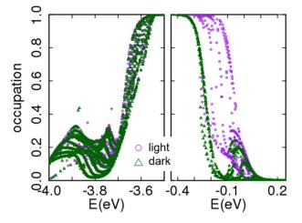
Figure 1: Hole (left) and electron (right) occupancy functions in the quantum well of Fig.1 at the position of 4.6nm with (purple) and without (green) light illumination. The carrier generation leads to an increase in hole and electron occupancy. The higher density of states in the valence band weakens the observed occupancy increase compared to the electrons in the conduction band.
