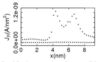
Figure 3: Recombination current density of the quantum well of Fig.1. The atom type, the quantum mechanical confinement and nonequilibrium occupancy determine the effective Büttiker probe recombination current.
