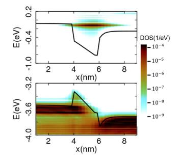
Figure 1: Density of states (contour) in the conduction band (above) and valence band (below) of a  $2nm GaN/In_{0.13}Ga_{0.87}N/GaN$  quantum well typical for blue light emitting diodes. Electrons enter from the left, holes from the right according to the p/n doping structure.
