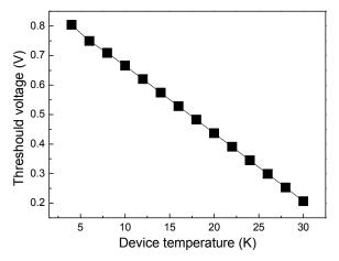
Fig. 3. Threshold voltage  $V_T$  of GaAs-based BIB detector as a function of device temperature  $T_{\text{Dev}}$ .
