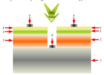
Fig. 1. Structural model of GaAs BIB THz detector.
