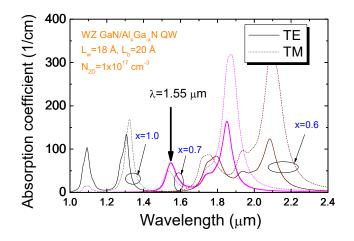
Fig. 2. TE(solid line)- and TM(dashed line)-polarized absorption spectra of (0001)-oriented wurtzite GaN/Al<sub>x</sub>Ga<sub>1-x</sub>N QW structure ( $L_w = 18$  Å,  $L_b = 20$  Å) with several Al contents in the barrier.
