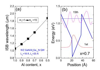
Fig. 1. (a) Intersubband transition wavelength as a function of Al content in the barrier for the absorption from the first subband  $(m_1=1)$  to the 15th higher subbands  $(m_2 = 15)$  of (0001)-oriented wurtzite GaN/Al<sub>x</sub>Ga<sub>1-x</sub>N QW structure with  $L_w = 18$  Å and  $L_b = 20$  Å and (b) potential profile and the wave functions for 1st and 15th subbands at zone center for the QW structure with x=0.7.
