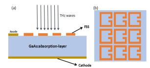
Fig. 1. Diagram of the GaAs device with periodic split-ring-shaped array.
