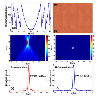
Figure 1: Rotation angle of the nanoblocks along x axis for on-center focusing. (b) Top view of the center of the reflective metalens. The required phase is imparted by rotating the nanoblock with different angle  $\theta(x,y)$ . (c) and (d) Simulated intensity (|E|2) profile of the reflected light in x-z plane at y=0 and in x-y plane at z=20 $\mu$ m with RCP incident light. (e) and (f) Vertical cuts of focal spot for the metalens with Au ground plane and PEC ground plane.
