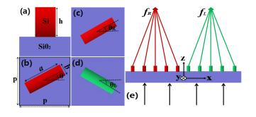
Figure 2: (a) Side view of the unit cell which composed of a silicon nanoblock placed on a half infinite silica substrate. (b) Top view of the unit cell. (c) and (d) The red and green nanoblocks with rotation angles  $\theta R$  and  $\theta L$  endow the required phase shift for focusing RCP and LCP lights, respectively. (e) Schematic of the metalens with RCP and LCP lights are focused into two focal spots.
