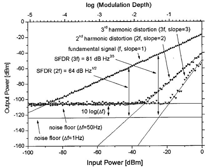
Fig. 4. Measured ac output power at different frequencies ( $f$ ,  $2f$ ,  $3f$ ) versus ac input power and modulation depth (dc current 4 mA, modulation frequency 1 GHz). Lines illustrate the extraction of the spurious-free dynamic range SFDR for second- and third-order harmonic distortion.
