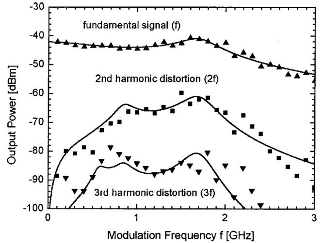
Fig. 3. Fundamental modulation response and harmonic distortions versus modulation frequency with 2.5-mA dc input current and 0.01 current modulation depth (dots: measurements; lines: calculation).
