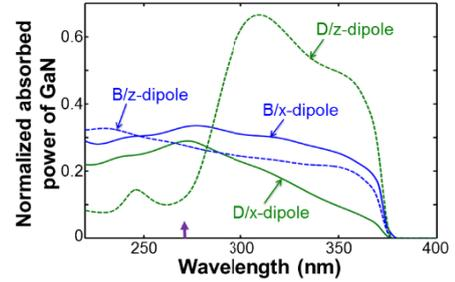
Fig. 3. Spectra of the normalized absorbed power of the GaN layers in structures B and D when either an  $x$ - or  $z$ -dipole at  $(x, y, z) = (0, 0, -a)$  is used.
