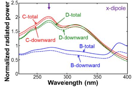
Fig. 2. Spectra of the normalized radiated power in structures B-D when an  $x$ -dipole at  $(x, y, z) = (0, 0, -a)$  is used. The vertical arrow marks 270 nm.
