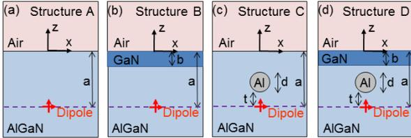
Fig. 1. (a)-(d): Schematic demonstration of the four simulation structures (A-D). The center of the Al NS in structure C or D is located at  $(x, y, z) = (0, 0, t + d/2 - a)$ .
