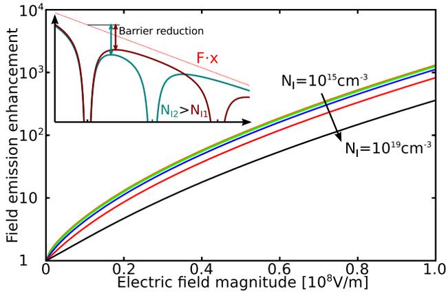
Fig. 1. Electric field related emission rate enhancement as a function of the electric field and the impurity density. The inset illustrates the barrier reduction at different impurity densities but the same electric field
