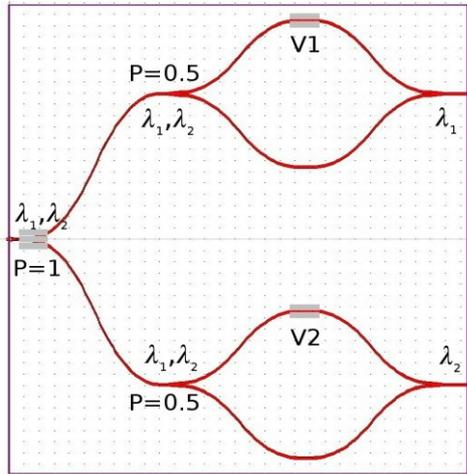
Fig. 1. Schematic design of an active reconfigurable node.
