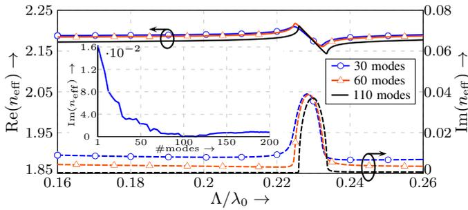
Fig. 2. Real part (solid lines) and imaginary part (dotted lines) of the fundamental mode effective index in the subwavelength grating waveguide for different numbers of eigenmodes used in the simulation. Inset: imaginary part of  $n_{\text{eff}}$  over the number of included modes for  $\Lambda/\lambda_0 = 0.1935$ .
