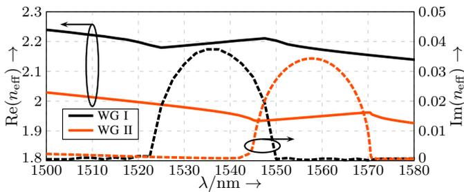
Fig. 3. Spectral characteristics of the real and imaginary part of  $n_{\text{eff}}$ . Waveguide parameters are  $\Lambda = 350$  nm and  $FF = 0.5$  (WG I),  $\Lambda = 400$  nm and  $FF = 0.41$  (WG II).
