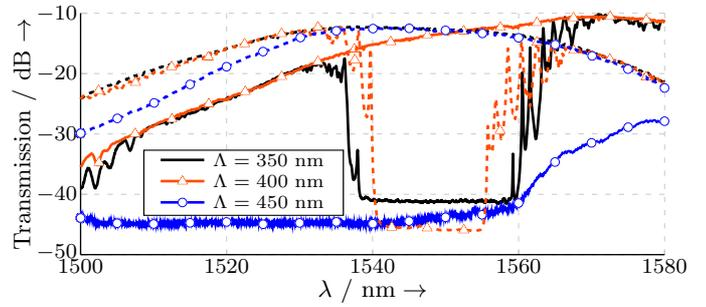
Fig. 4. Measured transmission spectra of waveguides without (solid curves) and with (dotted curves) oxidation step for different grating periods.
