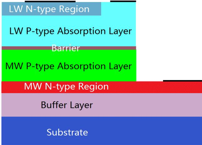
Fig. 1 Schematic of simultaneous two-color HgCdTe MWIR/LWIR detector investigated.
