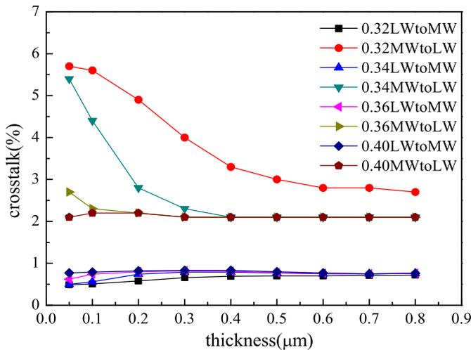
Fig. 5 Crosstalk as a function of  $d$  for different  $x$ 's
