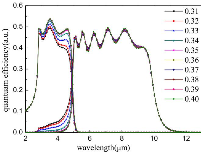
Fig. 3 Quantum efficiency related to  $x$  with  $d$  fixed at  $0.2\mu\text{m}$ .
