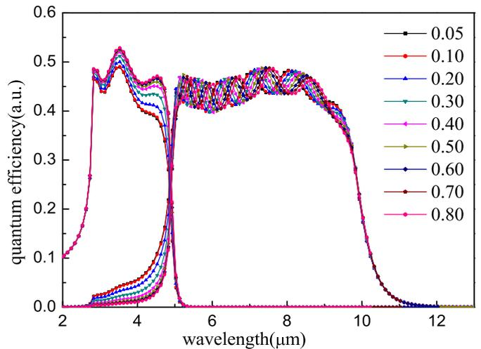
Fig. 4 Quantum efficiency related to  $d$  with  $x = 0.32$
