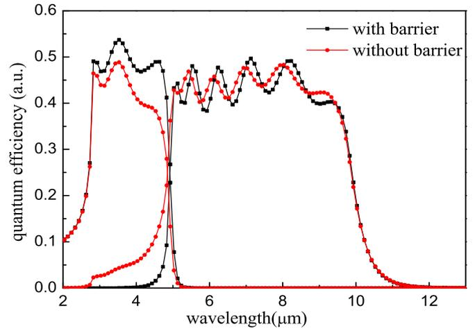
Fig. 2 Comparison of quantum efficiency between detectors with and without barrier.
