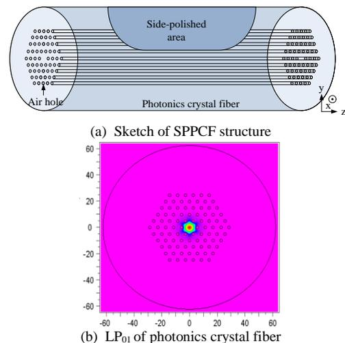
Fig.1. Sketch of SPPCF structure and LP<sub>01</sub> of photonics crystal fiber
